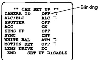
The CAM SET UP menu appears on the monitor as shown above.
