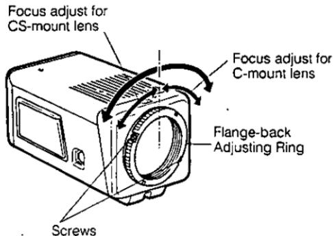
3. Tighten the screws on the flange-back adjusting ring.
