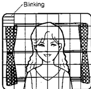
3. Move the cursor to the area where backlight is bright, and press
