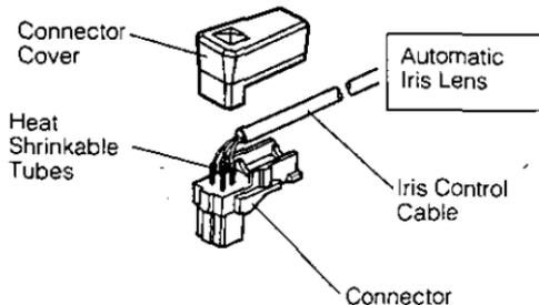
**Note:** When the iris control cable is too thick to lock the connector cover with the connector base, cut off the rib on the connector. (Select VIDEO for LENS DRIVE of the CAM SET UP menu.)
