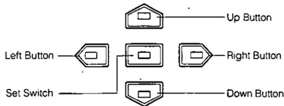
**Up Button (⏶):** This button is used to move the cursor upwards. Use this button to select an item or adjust the parameters.
